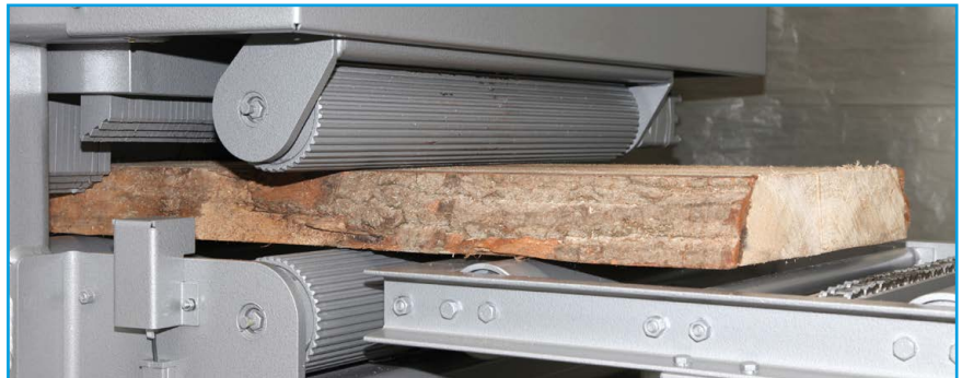
Fig. 19: Infeed pinch roller unit
