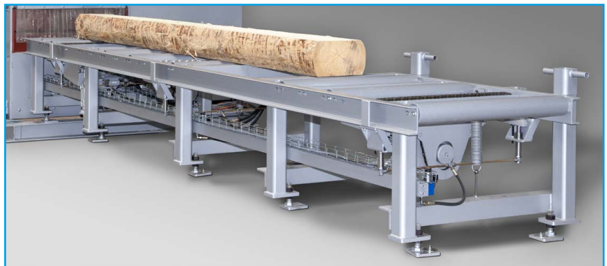
Fig. 18: Convenient alignment table, manually loaded
