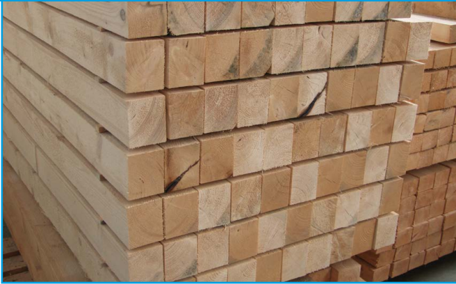
Fig. 6: Excellent cut finish on square timber ...
