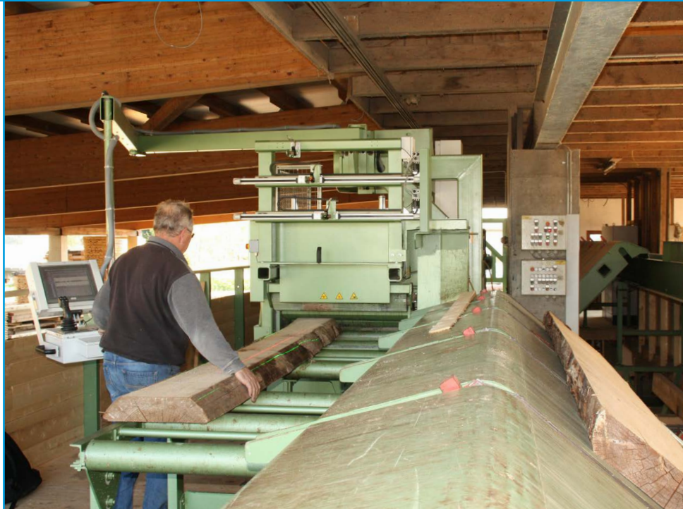
Fig. 2: KME3-1016, manually loaded, operating in a sawmill
