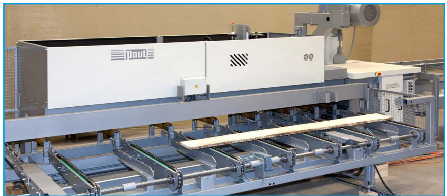
Fig. 17: AB920 fully automatic infeed system
