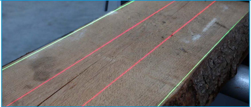
Fig. 16: Line lasers for ease of workpiece alignment
