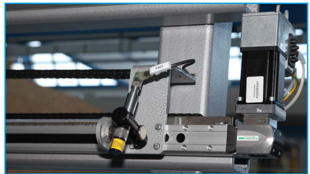
Fig. 12: Line lasers indicating the saw blade positions
